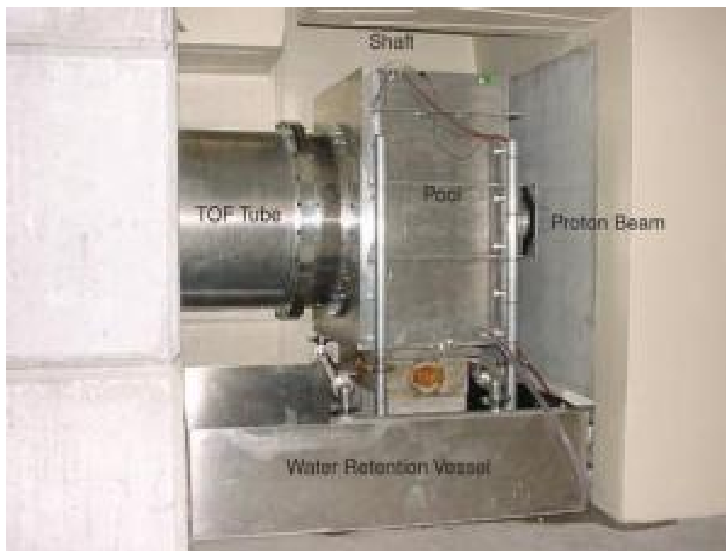
Labeled equipment in n_TOF facility. The n_Tof facility is operative at CERN (Genf), and is suitable for measuring the reactions of radioactive materials when bombarded with neutrons. (Credit: Image courtesy of Vienna University of Technology)
